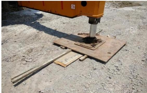
Gambar 3. 12 Proses *Jacking* Pada *Mobile Crane*
