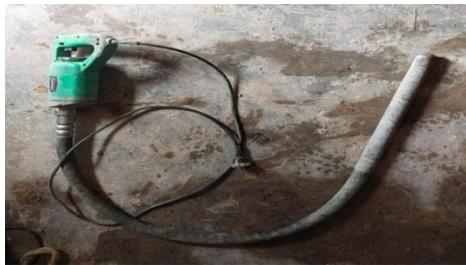
Gambar 2. 20 Concrete vibrator
