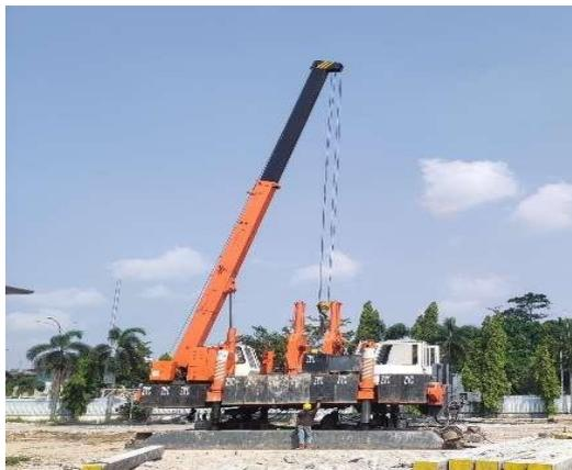
Gambar 2. 16 HSDP (Hidrolic Static Pile Driver)
