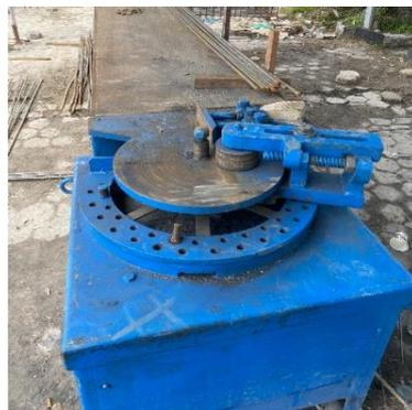
Gambar 2. 18 Bar bending
