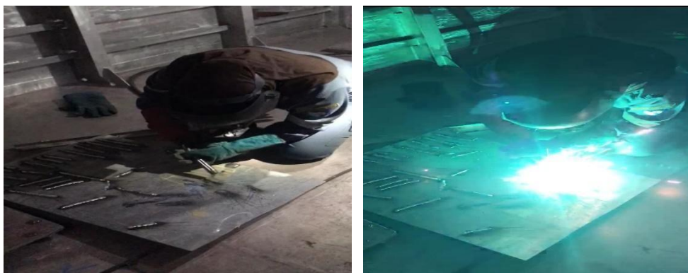
Gambar 3.21 proses pengelasan FCAW
