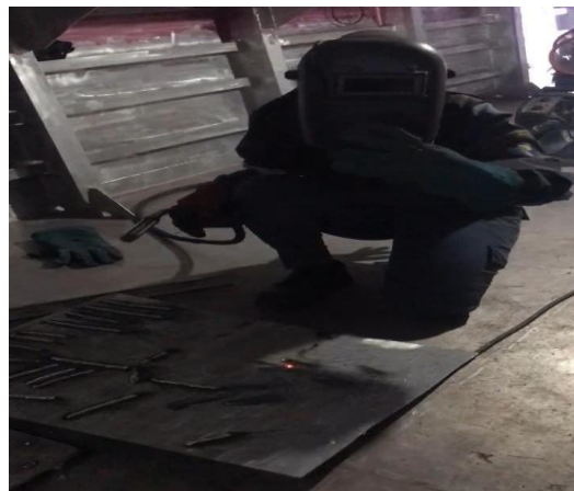
Gambar 3.22 proses pengelasan FCAW
