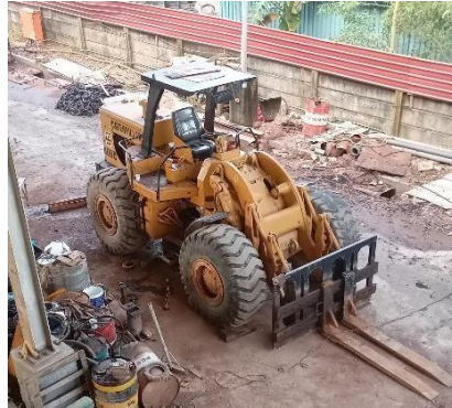
Gambar 2. 15 forklift Wheel Loader
