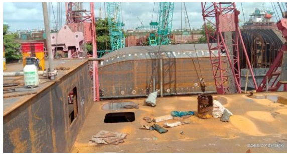
Gambar 3. 32 proses lifting turning up body
