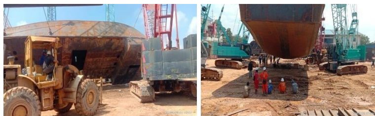
Gambar 3. 42 proses lifting turning up body
