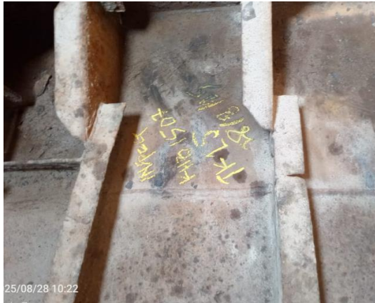
Gambar 3. 61 Welding Inspct Tangki Tongkang
