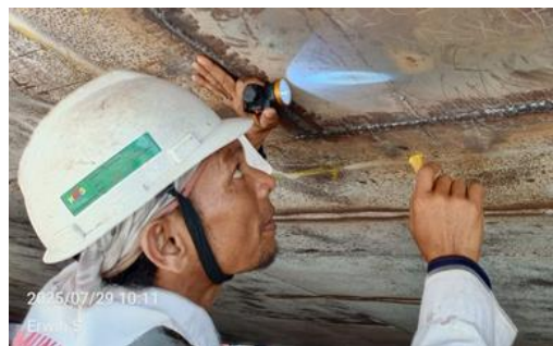
Gambar 4. 4 Marking Proses Vacuum
