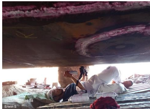
Gambar 4. 6 Proses Peneran Test
