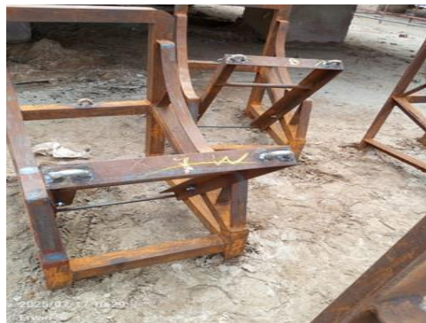
Gambar 3. 10 Welding Inspect Life Craft
