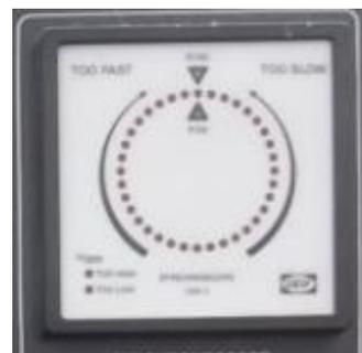
Gambar 4. 15 Synchronscope
