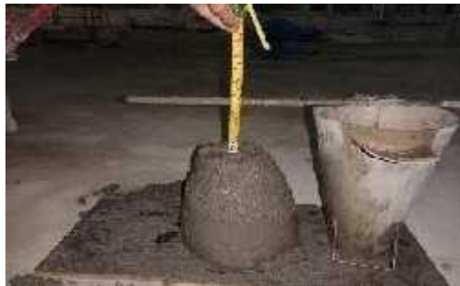
Gambar 2. 7: Pengujian Slump Beton
