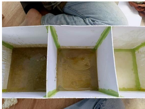
Gambar 4. 8 Pengujian OWS( Oil Water Separator)
